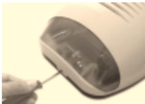
2) open the metal protection by unscrewing the two screws
