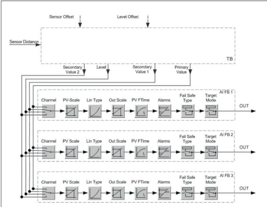
Figura 58: VEGAPULS 61: Block diagram with AI FB 1 ... AI FB 3 OUT values
