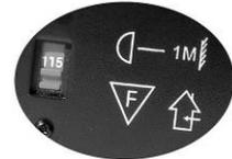
Not all fixtures have a voltage select switch. Please be sure to connect to the proper voltage.
