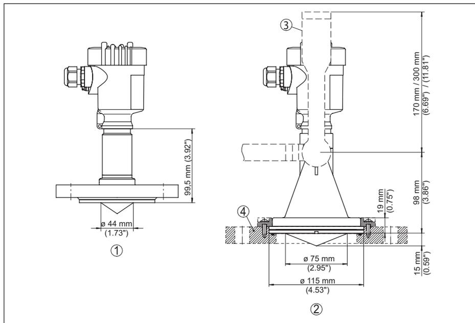
Figura 47: VEGAMIP 62, antenne incapsulate
