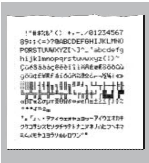
The LC-P43 is equipped with a self-test which automatically prints out the character set of the printer.
