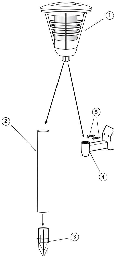
A flathead screwdriver is required for mounting the wall bracket.
