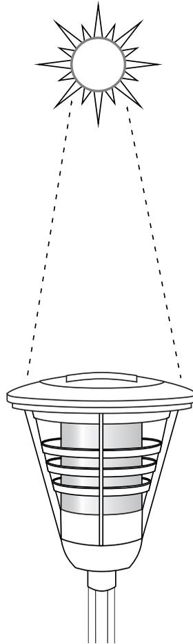
**BEFORE FIRST USE – Pull out to remove the clear plastic strip with orange sticker in the light fixture to charge battery.**
