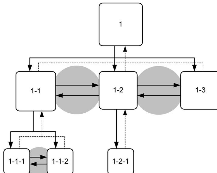
**Figure 4-3.** In this example, each displayed state is a folder containing a list of items. State one contains three folders (1-1, 1-2, 1-3). When the user has opened one of these, there is a possibility to move directly into the other two folders without first going back to state 1. Folder 1-1 contains two sub-folders and folder 1-2 contains one. There can be individual items in each folder in addition to the folders; those are not visible in the state diagram.
