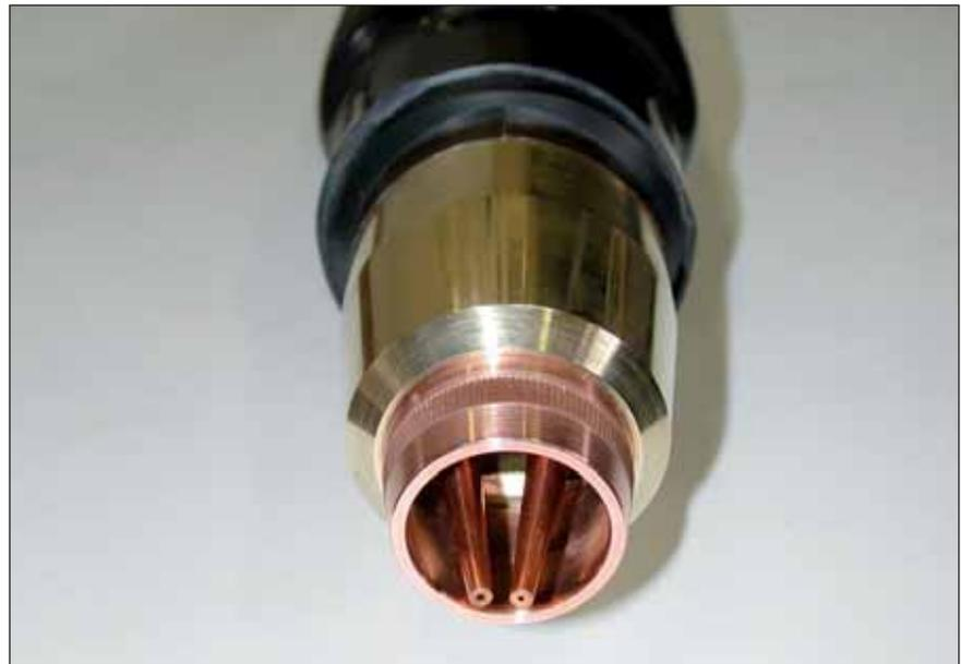
Figure 1 - Water cooled tandem welding torch designed for narrow groove welding.
