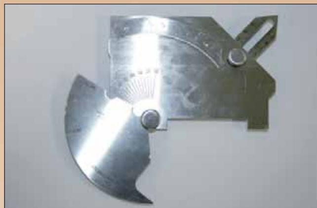
Figura 3b - Multi-Purpose Gauge - Side B.
