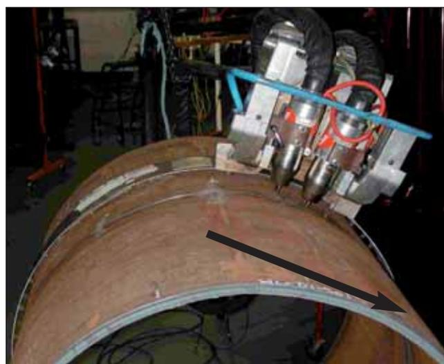
Figure 3 - Double jointing weld procedure configuration.
