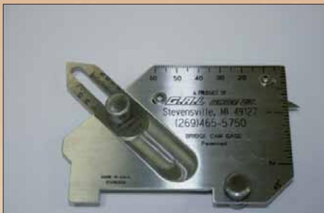
Figura 3a - Multi-Purpose Gauge - Side A.
