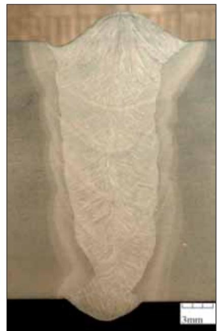
Figure 5 - Dual tandem double jointing procedure macro section.
