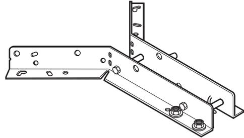
Y-Brackets not required with steel-framed acrylic boards. Remove them before beginning assembly.
