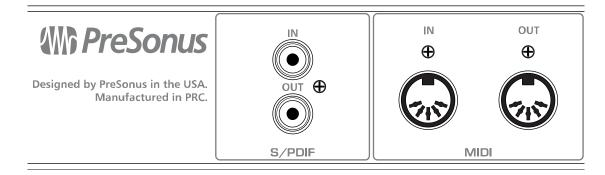
• S/PDIF In and Out Jacks. These allow the FireStudio Project to receive and transmit audio from other digital audio devices. The S/PDIF standard allows two channels of audio to be transmitted at rates up to 24bit/96kHz. The S/PDIF input also allows the FireStudio Project to receive Word Clock – the synchronizing signal indicating the sampling frequency or rate of sample words over a digital interface.
