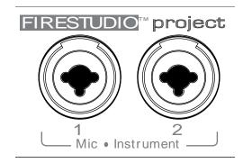
• Instrument Inputs (Channels 1 and 2). The ¼" TS connector on channels 1 and 2 are for use with an instrument (guitar, bass, etc.). When an instrument is plugged into the instrument input, the microphone preamp is bypassed, and the FireStudio Project becomes an active instrument preamplifier.
