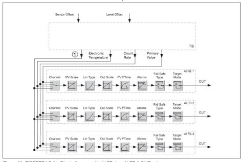
Figura 23: FIBERTRAC 31: Block diagram with AI FB 1 ... AI FB 3 OUT values
