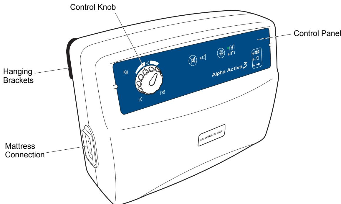
The controls are situated on the front of the pump. An alarm system differentiates between normal operation and genuine system faults. If an alarm situation is detected an indicator will illuminate on the front of the pump and an audible warning will sound.
