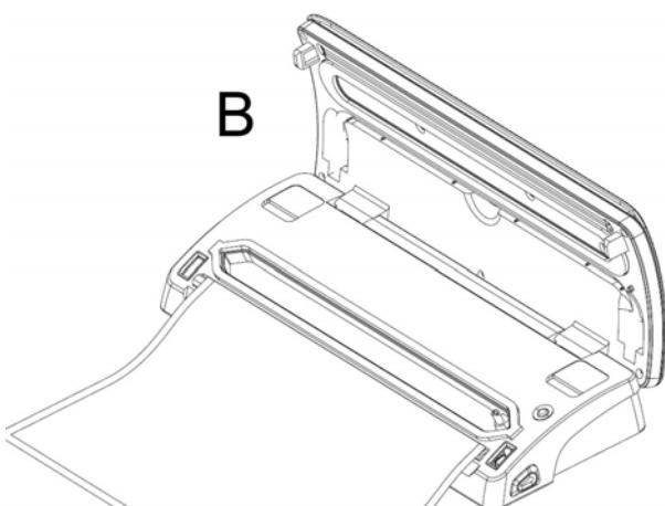
2. Put one end of the bag on top of the sealing profile (4) and the lower gasket (6) The open end of bag must not enter the vacuum chamber (5) (image B).
