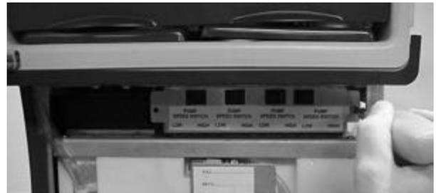
3. Pull the electrical box forward and straight out.
