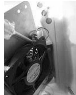
4. Remove (4) screws from the fan mounting bracket.
