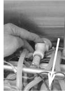
6. Disconnect the platform electrical connector by squeezing the release tabs on either side of the connector and pulling straight back. The platform can now be removed from the cabinet.
