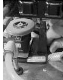
2. Lift the motor out of the ice bath. Disconnect the wire lead from the ice bank control.
