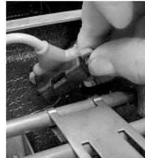
2. The connector must be disassembled to pass the wire leads through the water bath cover.
