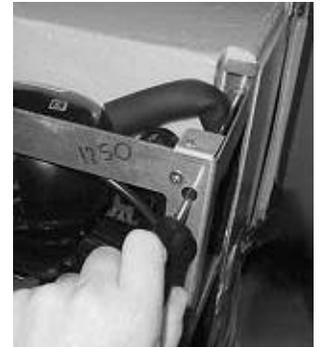
8. After you lift the cabinet off the frame you can service the agitator motor.
