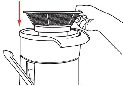
4. Place the juicer cover onto the juice collector / bowl, with the feed chute positioned over the stainless steel blade and filtering basket and push into position – figure 4.
