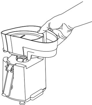
2. Place the juice collector / bowl onto the top of the motor base.
