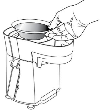
4. Place the juicer cover onto the juice collector / bowl, with the feed chute positioned over the stainless steel blade and filtering basket and push into position.
