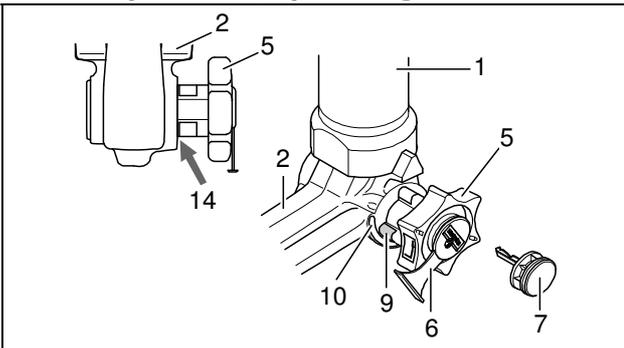
**Unlocked position, ball bar not mounted**
