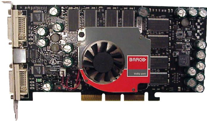
Figura 4: The BarcoMed 2MP2CF-3D display controller
