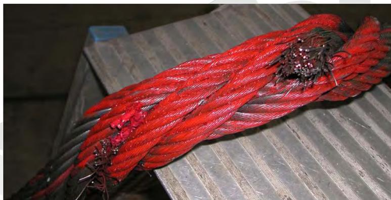
Cable-laid slings of different lay directions should never be joined together
