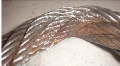
The competent person should consider measuring the actual length of the cable-laid sling or grommet, and the lengths of the splice tails, as these can give an important indication of serious deterioration.
