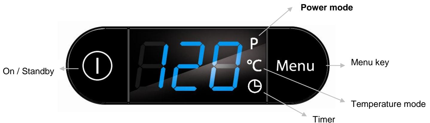
The display is used to show the selected temperature, power level, timer and to show the error code in the event of a malfunction.
