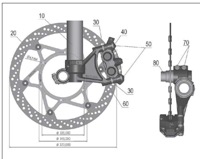
The distance sleeve (80) is also necessary for the 660 models (2003, 2004, 2005) and 640 supermoto (2005), since the fork bridges with distance dimensions and hubs are used which differ from the standard, additional distance rings are available with thicknesses of 2.5 and 4.0 mm for the KTM brake discs.
