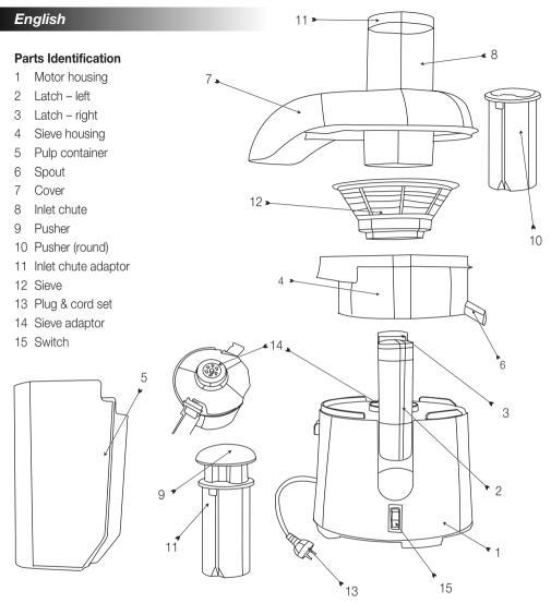
**Note:** The Juicer will not operate unless all the parts (pulp container (5), sieve housing (12), latches (2,3) and cover (7)) are correctly fitted.
