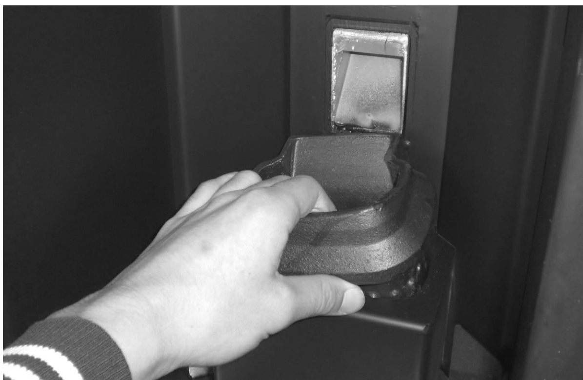
Carefully clean the brazier from combustion residues, by removing it from its seat.
