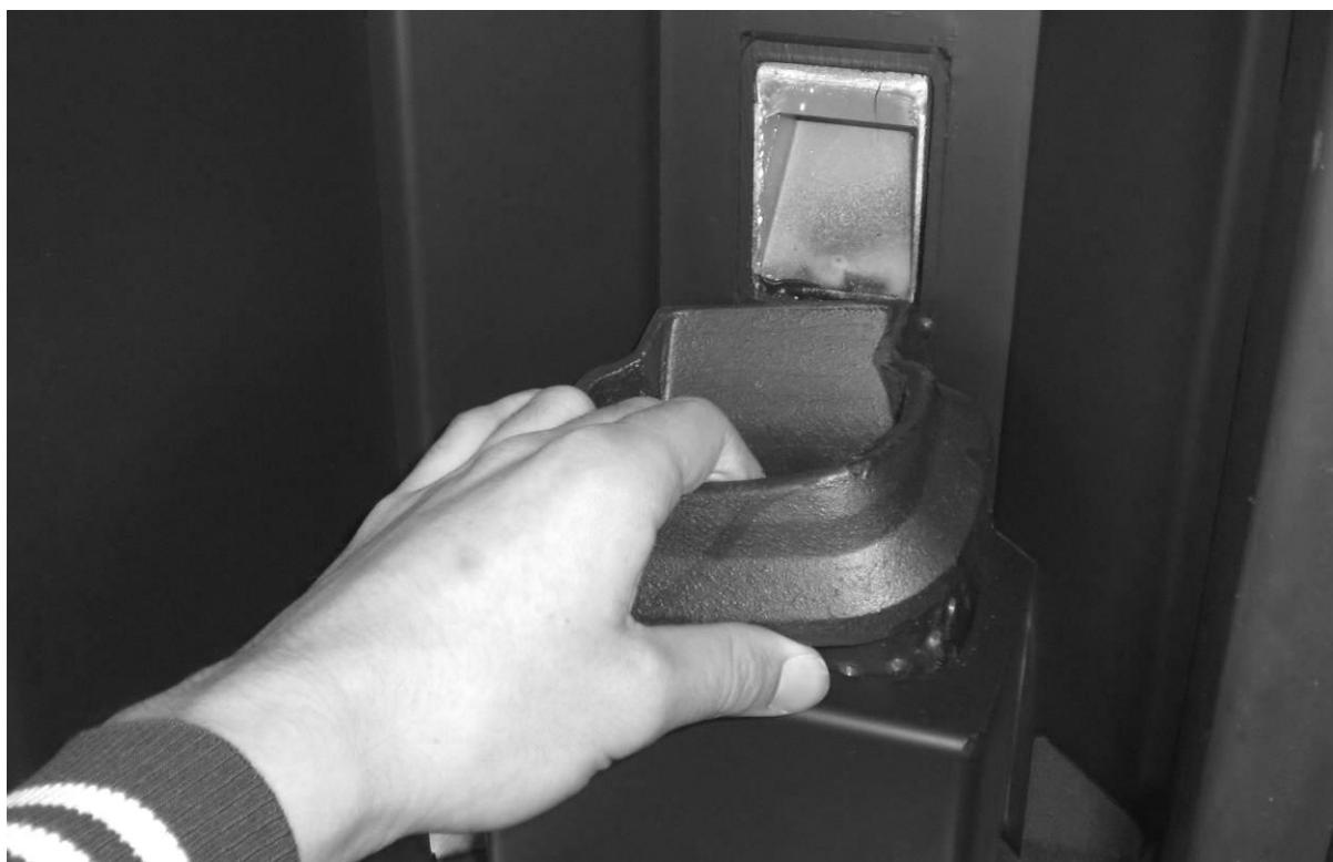
Carefully clean any combustion residues from the brazier, by removing it from its housing.
