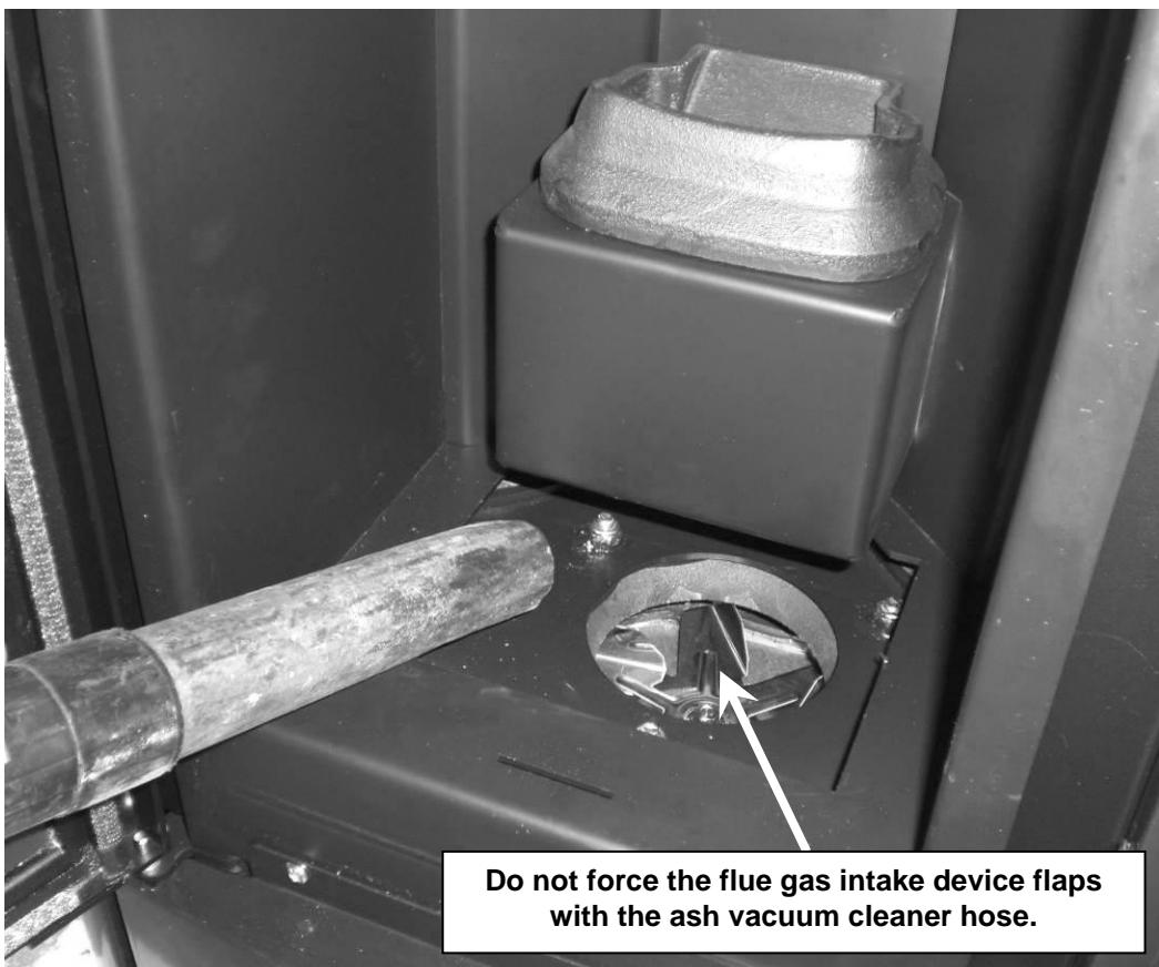
Use a suitable ash vacuum cleaner to remove the internal residues then re-position the base and ash drawer.
