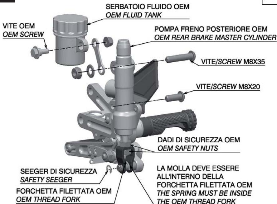
PART NUMBER **PER318** MONTAGGIO SWITCH LUCE STOP OEM *INSTALL OEM STOP LIGHT SWITCH*
