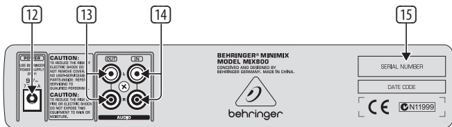
Fig. 2.2: Rear panel connectors of the MIX800
