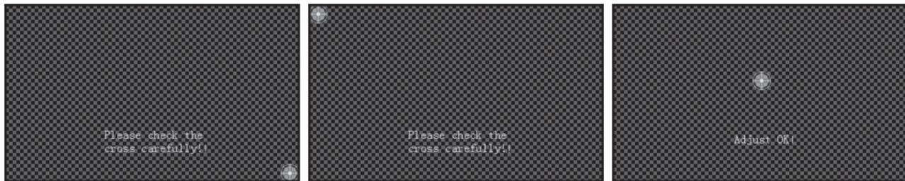
*The text on the first two calibration screens advise you to “Please check the cross carefully” with the Stylus. The final screen reads “Adjust OK” after you have successfully clicked your way through.*
