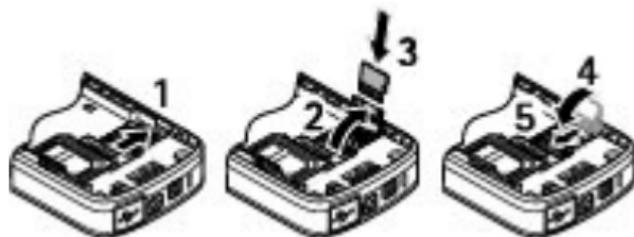
1. Switch the phone off, and remove the back cover and the phone battery.
