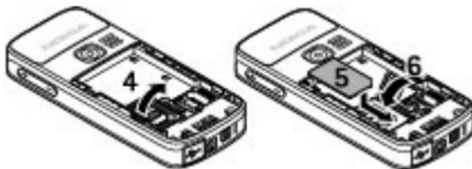
contacts (7), and insert the battery (8). Place the upper part of the back cover on the device (9), and close it (10).
