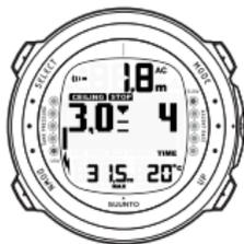
QUANDO IL DISPLAY INDICA CEILING E STOP CON UNA FRECCIA RIVOLTA VERSO IL BASSO, SCENDERE IMMEDIATAMENTE (ENTRO 3 MINUTI) AL LIVELLO DEL CEILING O A UNA PROFONDITÀ MAGGIORE.
