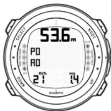
ATTIVAZIONE MODALITÀ NITROX DIVE (IMMERSIONE CON NITROX). MASSIMA PROFONDITÀ OPERATIVA IN BASE ALLA % DI O<sub>2</sub> IMPOSTATA (21%) E AL VALORE DI PO<sub>2</sub> (1,4 BAR): 53,6 M.
