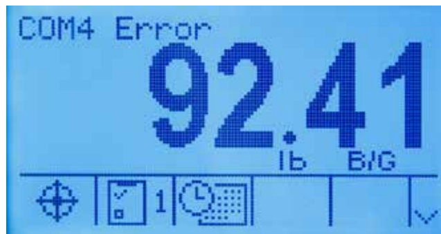
Figura 4-2: COM4 and COM5 Communication Errors
