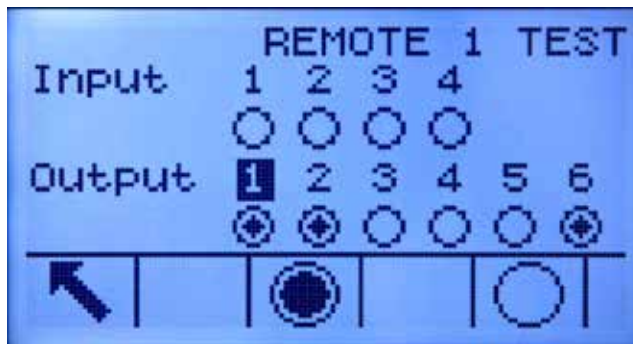
Figura 4-5: Schermata Test I/O discreti
