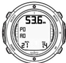
ATTIVAZIONE MODALITÀ NITROX DIVE (IMMERSIONE CON NITROX). MASSIMA PROFONDITÀ OPERATIVA IN BASE ALLA % DI O<sub>2</sub> IMPOSTATA (21%) E AL VALORE DI PO<sub>2</sub> (1,4 BAR): 53,6 M.
