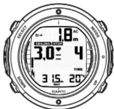
QUANDO IL DISPLAY INDICA CEILING E STOP CON UNA FRECCIA RIVOLTA VERSO IL BASSO, SCENDERE IMMEDIATAMENTE (ENTRO 3 MINUTI) AL LIVELLO DEL CEILING O A UNA PROFONDITÀ MAGGIORE.
