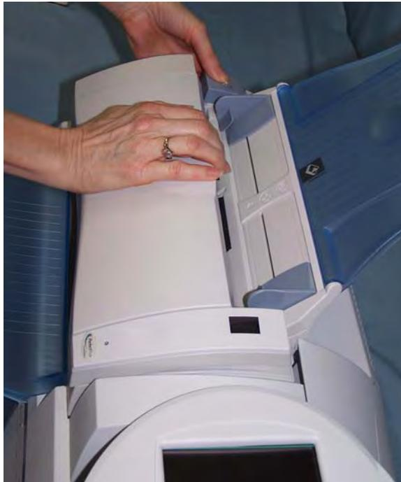
2. When finished with the cleaning procedures, close the Scan Station cover.
