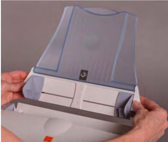
2. Align the input tray pins with the slots.
