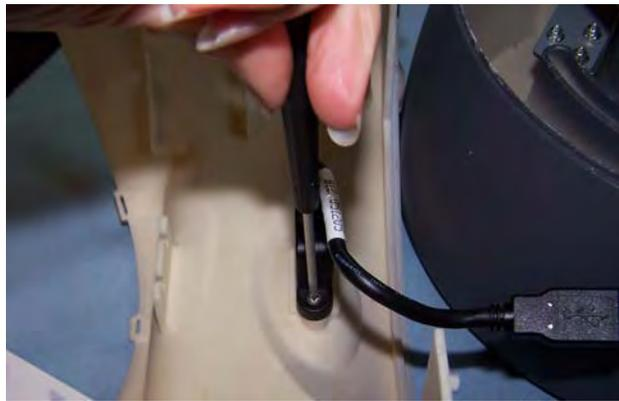
11. Attach the new USB cable to the connector and tighten the screws.
