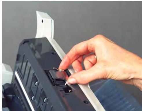
2. Wipe the feed module from top to bottom with a roller cleaning pad.
