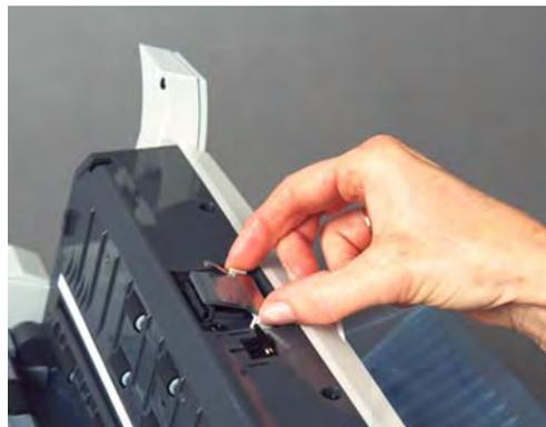
3. Insert the new feed module into position, aligning the new module into the slots, and pushing it in until it snaps into place.
