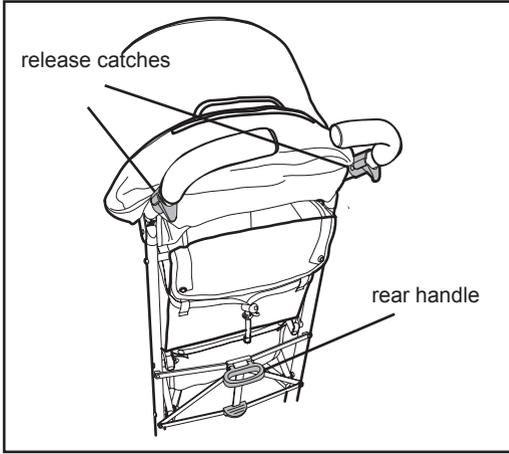
To fold your pushchair pull the rear handle upwards till the pushchair begins to fold - DO NOT FORCE IT. Whilst pulling up on the release catches push the handles away from you folding the pushchair.
