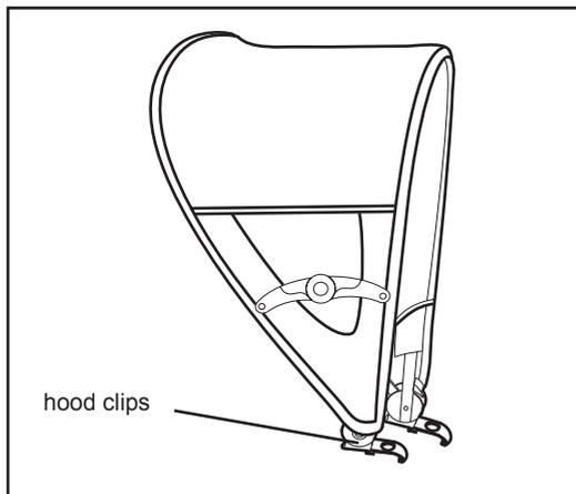
To attach the front hood: insert the hood clips into the slots on the pushchair arms as indicated below.
