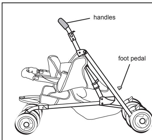
When nearly all the way up place your foot on the foot pedal and continue pulling the handles till the pushchair is fully erect.
