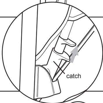
The rear seat has 3 recline positions. To lower the back rest lift the catches on both sides of the seat and position as required. To raise simply push the backrest forwards to the desired position.
