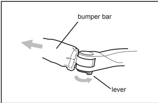
To open the bumper bar turn the lever to the right as indicated by the arrow. Whilst holding the lever in this position pull on the bumper bar to free it.
