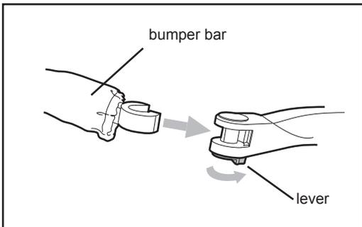
To close the bumper bar again, turn the lever to the right as indicated by the arrow and push the bumper bar back into place. Letting go of the lever will lock the bar safely in position.
