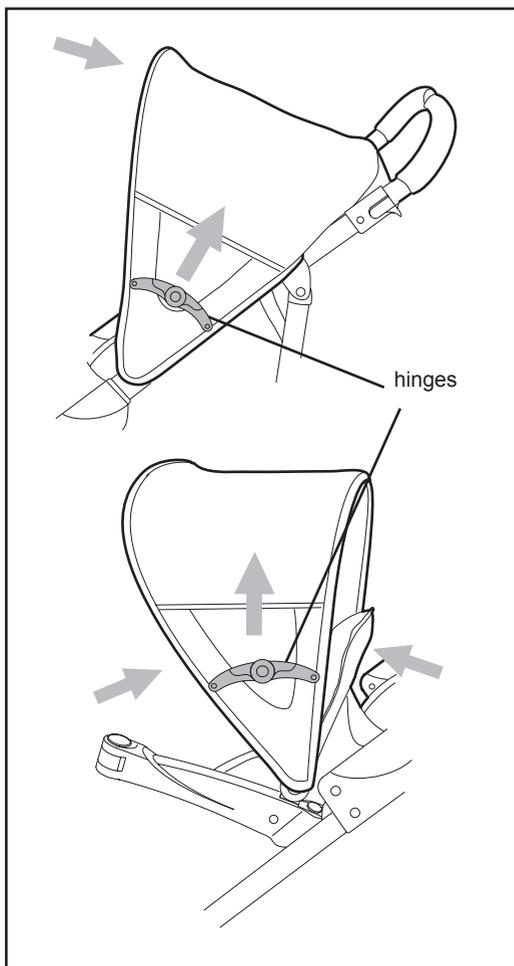
Both hoods can be folded back by lifting the hinges on either side of each and pushing the hood frame backwards.
