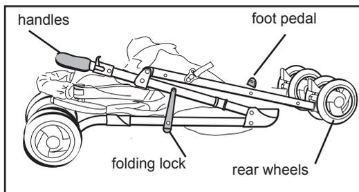
In order to unfold your pushchair first release the folding lock. Next hold the pushchair firmly by both handles and with a foot placed behind the rear wheels pull the handles upwards towards you.
