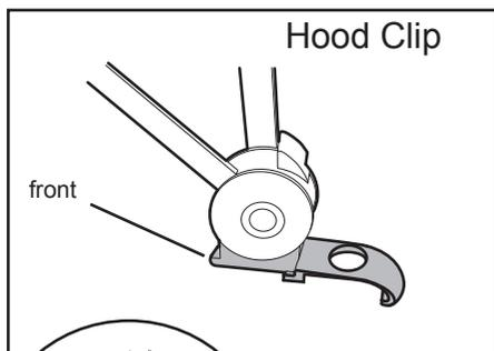
Holding the hood clips at a slight angle insert the front of each hood clip into the slot on the pushchair arm, then push down and forward to secure.
