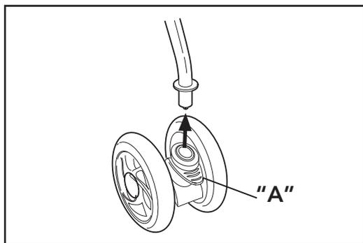
To fit the front wheels, push each wheel assembly on to the front legs, ensuring that they engage securely.
