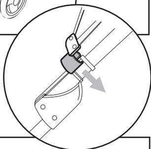
Holding the hood clips, twist them slightly to allow ease of attachment to the pushchair frame.
