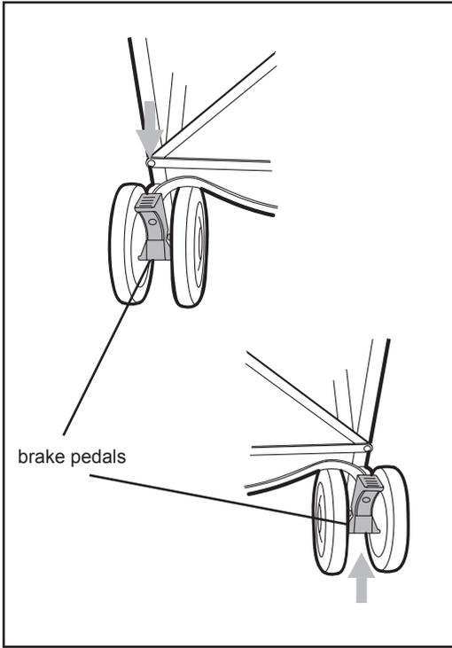
Using your foot, push down on either brake pedal till the mechanism clicks into place, engaging the brakes. Check the brakes are securely engaged by gently pushing forwards against the pushchair handles.
