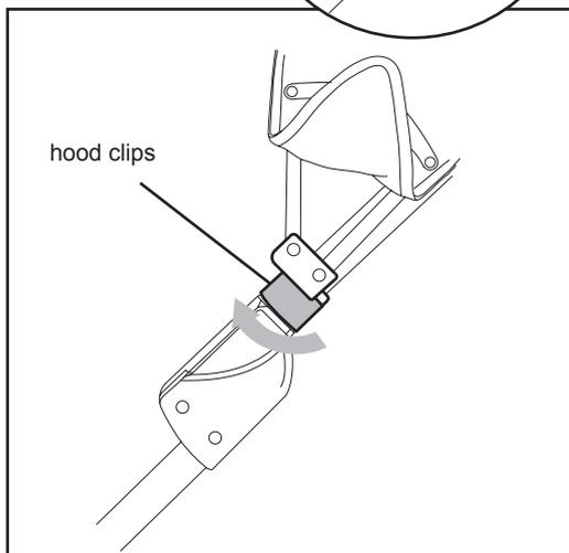
To detach: twist the hood clips slightly inwards towards the centre of the pushchair then remove from the chassis.
