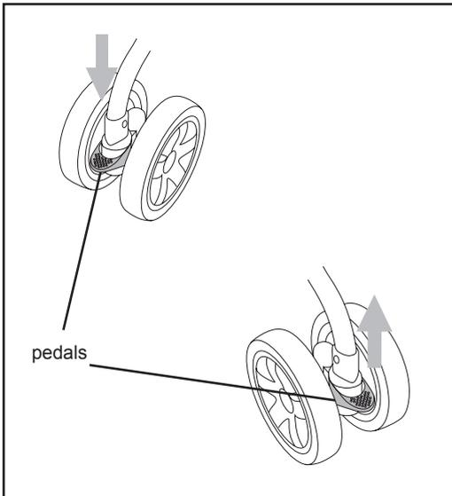
Your pushchair is equipped with lockable swivel wheels. To lock the front wheels push down on both swivel locking pedals. To unlock: lift both pedals.
