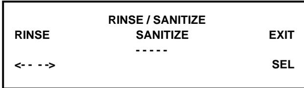
Pressing the MENU (SEL) key will give you the option to sanitize the left cylinder. Move the cursor under the word "YES". Pressing the MENU (SEL) key at this time will start the flow of cleaner/sanitizer through the syrup system into the freezing cylinder.
