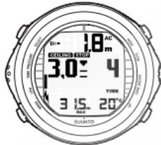
QUANDO IL DISPLAY INDICA CEILING E STOP CON UNA FRECCIA RIVOLTA VERSO IL BASSO, SCENDERE IMMEDIATAMENTE (ENTRO 3 MINUTI) AL LIVELLO DEL CEILING O A UNA PROFONDITÀ MAGGIORE.
