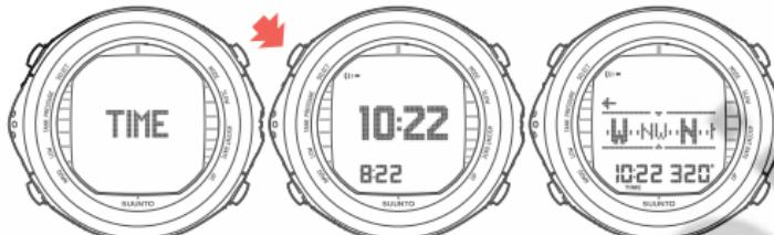
SE SI ACCEDA DALLA MODALITÀ TIME, NELLA PARTE INFERIORE DELLO SCHERMO SONO VISUALIZZATI IL TEMPO E IL RILEVAMENTO.
