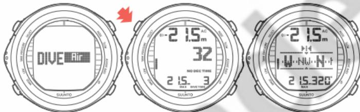
SE SI ACCEDA DALLA MODALITÀ DIVE, VENGONO VISUALIZZATE LA PROFONDITÀ E L'ORA CORRENTE O LA PROFONDITÀ MASSIMA, LA PRESSIONE DELLE BOMBOLE, IL RILEVAMENTO, IL TEMPO DI IMMERSIONE O LA TEMPERATURA.
