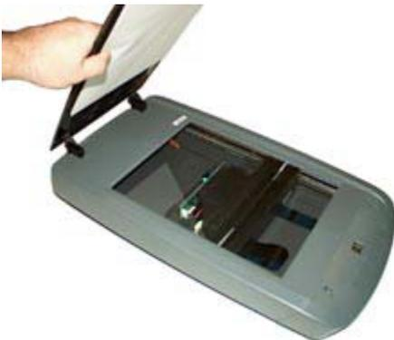
**scanner lid being re-inserted in scanner**
