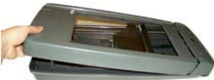
**top cover being installed onto base**
