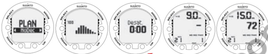
QUANDO SI ATTIVA LA MODALITÀ MEMPLAN, IL DISPLAY MOSTRA BREVEMENTE IL TEMPO DI DESATURAZIONE RIMANENTE (TISSUE LOADING) PRIMA DI PASSARE ALLA MODALITÀ PLAN. PREMERE I PULSANTI UP E DOWN PER SCORRERE NELL'ELENCO DEI DIVERSI LIMITI DI NON DECOMPRESSIONE. I LIMITI DI NON DECOMPRESSIONE SUPERIORI A 99 MINUTI SONO VISUALIZZATI CON IL SIMBOLO "—".
