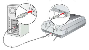
**Note:** Your scanner may not work correctly if you use a USB cable other than the one supplied by EPSON or if you connect your scanner through more than one hub.
