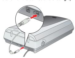
4 Connect either the USB cable that came with the scanner or an optional IEEE 1394 (FireWire) cable. **Do not connect both cables.**
