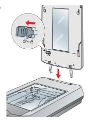
Attach the document mat. Hold the top of the document mat and slide it down gently along the document cover. Make sure the tabs on the bottom and sides of the document mat fit in the slots on the document cover.
