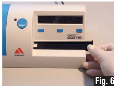
Fig. 6 Fig. 6 Correct handling of the strip holder for positioning it into the device after cleaning.
