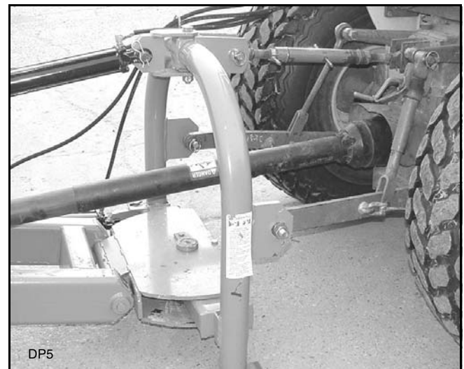
Figure 6. Stump Grinder Attached to Tractor (Category 1 Hitch Pins Shown)
