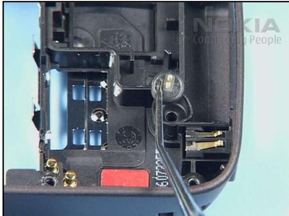
44. Remove the MICROPHONE with the dental pick.
