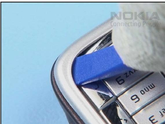
5. Place the SS-93 between the KEYMAT and the edge of the A-COVER and unlock the button clip first.
