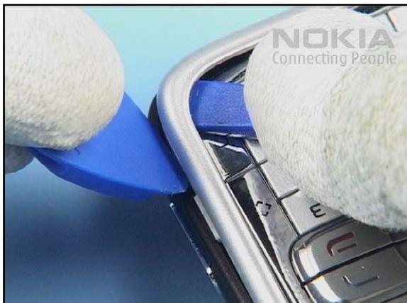
6. Hold the SS-93 in the shown position and unlock the side clip with SRT-6 by pressing it between the A-COVER and the B-COVER.
