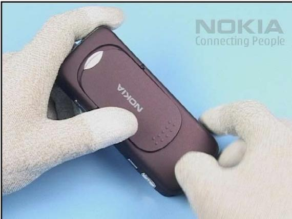
3. Unlock and open the SLIDE COVER ASSEMBLY.
