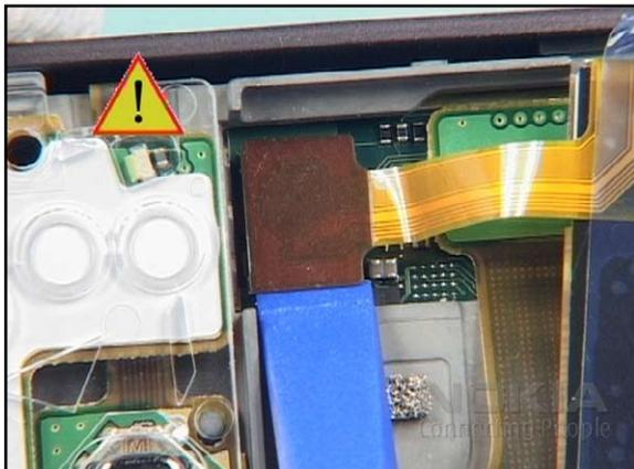
16. ...and disconnect it from the ENGINE MODULE.
