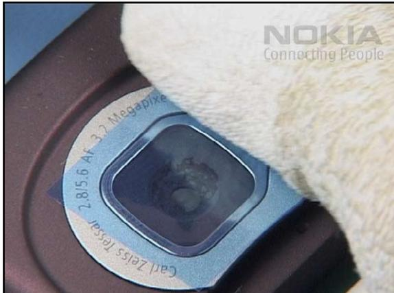
4. Cover the CAMERA WINDOW with a protective film.
