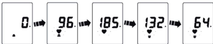
4 The blood pressure and pulse rate are displayed when the measurement completed.
