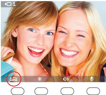
2) When an icon is shown, this means that a single P function activation has been configured
