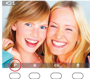
3) When the letter P is shown, this means that between 2 and 16 P function activations have been configured
