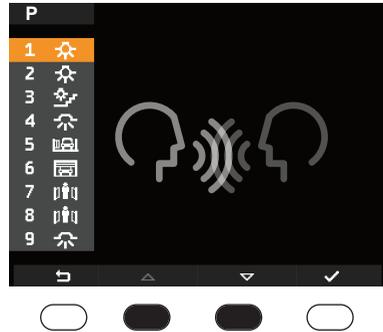
2) Buttons B and C are used to scroll through the menu to select the desired function
