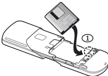
Press the battery down into the battery slot (2).
