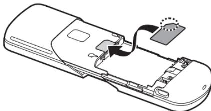
Replace the battery with the gold-coloured contact end aligned with the gold-coloured contacts in the battery slot (1).
