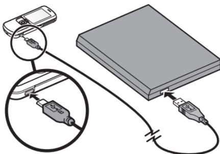
1. Connect the lead from the CA-101 to the micro USB socket on the lower right side of your phone.
