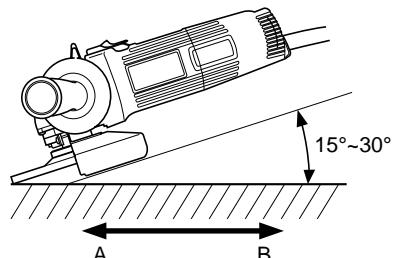
**NOTE:** The wheel provided (resinoid wheel) is rated as Class A grain and # 36 grain size. It is most suitable for heavy grinding of steel and other types of materials.
