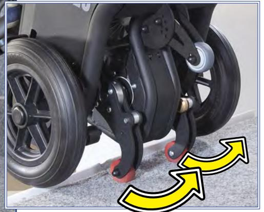
**D3** The arms rotate as indicated in the figure, while the aid is gradually pushed forwards and downwards
