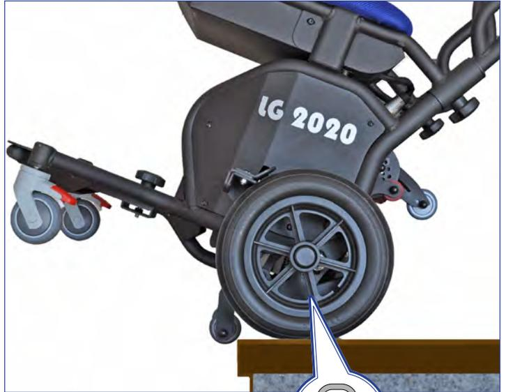
**D2** The arms rotate as indicated in the figure, while the aid is gradually pushed forwards and downwards
