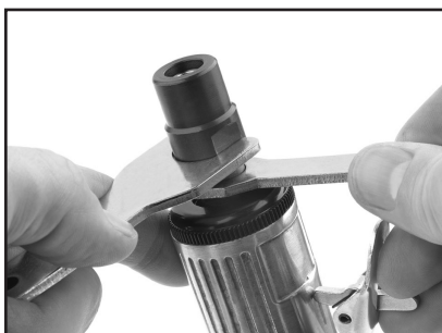
Figure 2. Loosening the collet.
