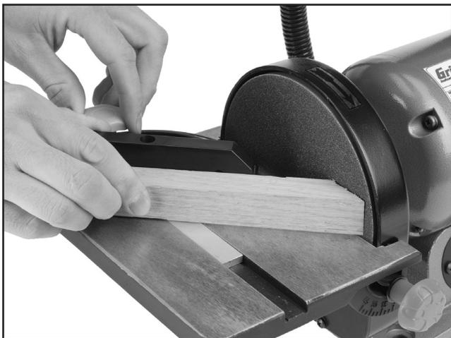
**Figure 12.** Disc sanding with a miter gauge.
