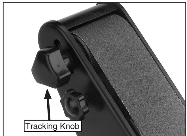
**Figure 10.** Sanding belt tracking knob.
