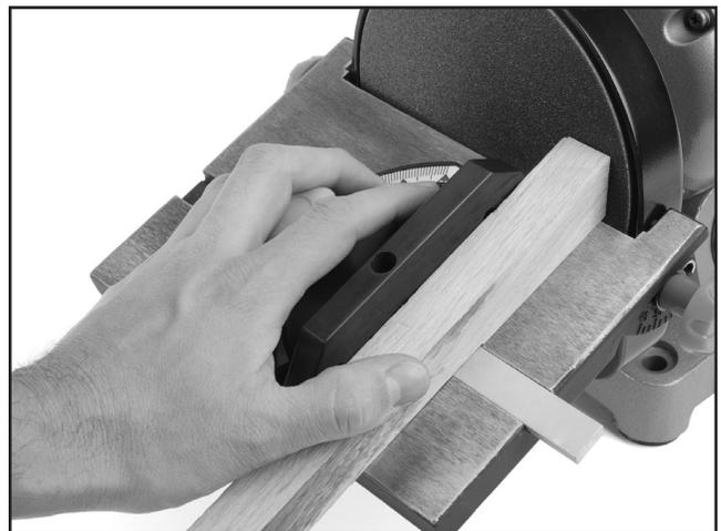
**Figure 13.** Mitering with the table angled.
