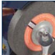
**Note.** The wheel on the left-hand side of the grinder has a left-hand thread and is unscrewed in a clockwise direction. The wheel on the right-hand side of the grinder has a right-hand thread and is unscrewed in an anti-clockwise direction.
