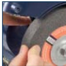
6. Replace the outer flange and retaining nut (see the Note above regarding the direction of rotation of the nut).
