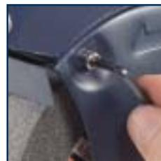
3. Slide the spark deflector up or down so that the bottom edge is less than 6mm from the surface of the wheel, but not touching the wheel.
