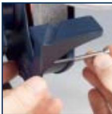
2. Hold the tool rest (10) in the correct position against the inner surface of the wheel guard. Fit the screw through both sides of the guard and then through the tool rest.
