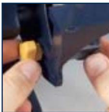
4. Slide the tool rest to within a maximum of 1.5mm from the wheel. Rotate the wheel one full revolution by hand to ensure the wheel does not contact the tool rest.
