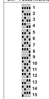
**NOTE :** if pulse average calculation is not required, leave all the **SW7** selector dip-switches **OFF** (shifted down).
